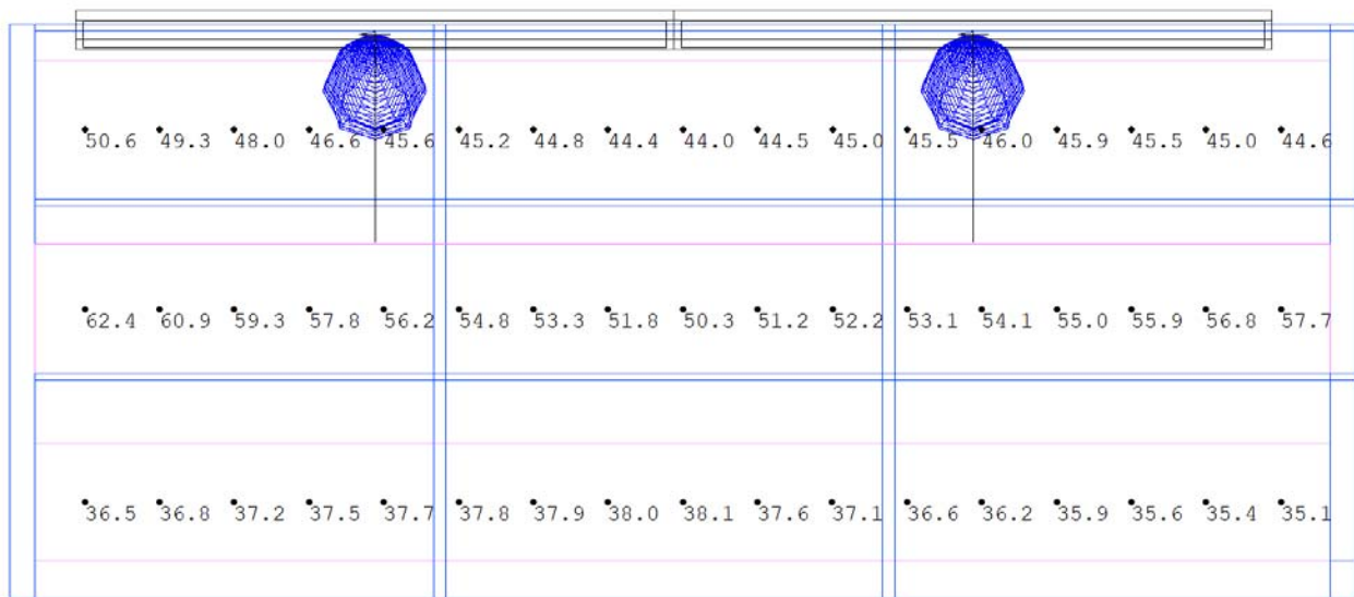
Above: Horizontal floor between shorter stacks, illuminance calculation Below: Shorter magazine stack, illuminance calculation
