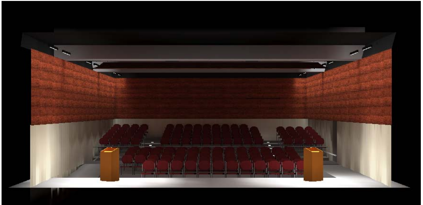
Above: Rendering looking at seating from stage view (Podium Speaker/Projection Scene –Overhead Lights Off, WallWashers 25%, step lights On, Accent lights on podiums only)
